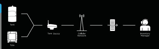
The 4000 Series Prophet UpLink, combined with TankData Online can help eliminate overflows and costly contaminations, and increase operations efficiency. Using a standard internet browser, you can retrieve and use valuable tank information virtually anywhere in the world, whether the tank is local or a thousand miles away. You'll make smart, data-driven decisions, anticipating operational needs and decreasing costs to operate.
